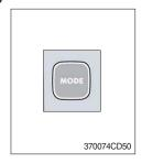
(1) Operating this switch, it beeps and displays symbol of each mode in order. (Vent → Vent/Foot → Def/Foot → Def/Vent → Def/Vent/Foot)
